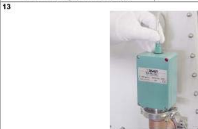
Insert measuring probe and re-clamp.
