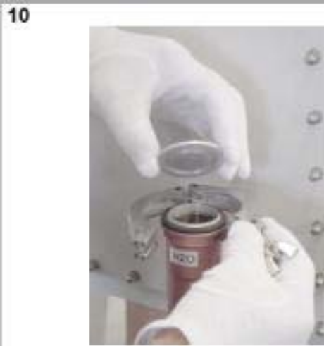
Remove clamp and dummy plug.
