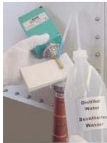
Moisten sensor with distilled water.
