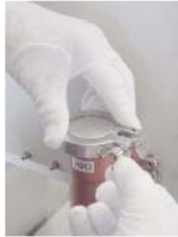
Tighten flange clamp.
