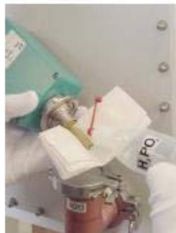
Moisten winding with phosphorous acid.
